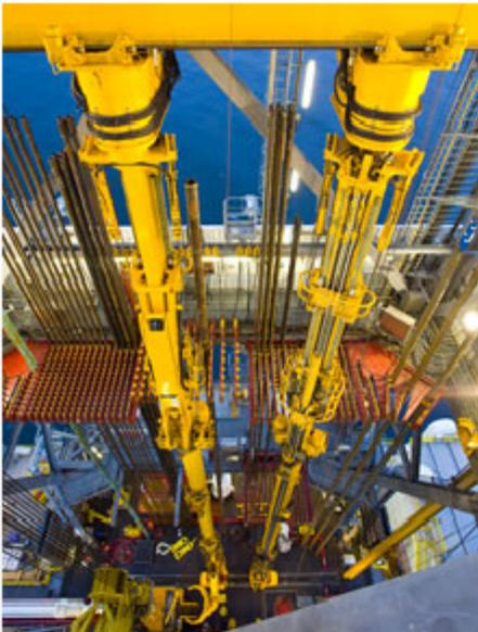
A deepwater drillship's pipe racking system.
