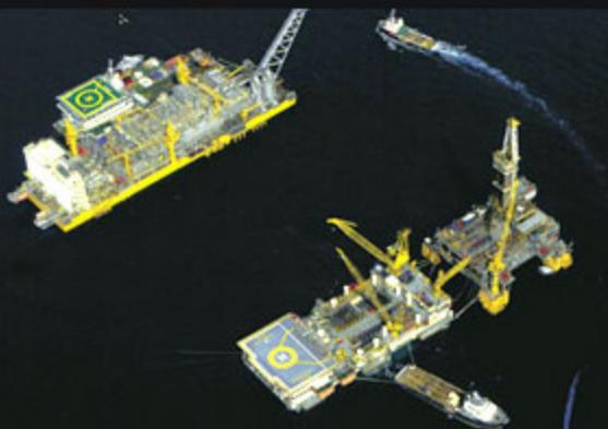
Our West Seno development in deepwater Indonesia features a hybrid of two platform types - the TLP connected to a floating production, storage and offloading vessel (see panel 6). Once built, our Papa Terra facility (part of a joint venture) in Brazil will be similar.
